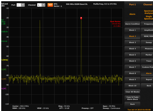
Figure 7: CW tone generation injected into the system to measure intermodulation
